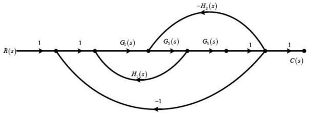
$$\begin{split} &\Delta_1 = 1 - 0 = 1 \\ &\Delta = 1 - \left(G_1(s)G_2(s)H_1(s) - G_2(s)G_3(s)H_2(s) - G_1(s)G_2(s)G_3(s)\right) + \left(0\right) - \dots \end{split}$$
